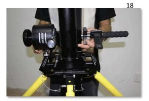
Connect the ropes via the carabineer clamp. The carabineer connectors make it very easy to attach and detach the handle from the tubes.
