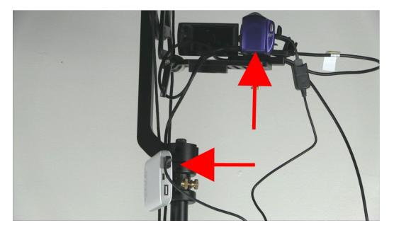
Find the USB power pack (exact style may vary but setup will remain the same), and attach to the tower where there is a hook at the top of the tubes. Use the brass screw (shown in the image) to sandwich the battery to the tower.
