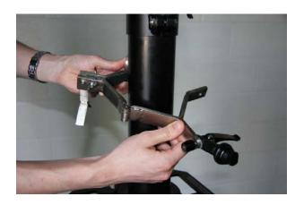
This LCD bracket is much easier to use than the previous one. Simply slide the hook into the back of the LCD monitor. Once you slide the hook into the slot, position it where you want it, then tighten down on it with the threaded screw. Now to position the LCD so it best for your viewing, loosen the camlock. Reposition and then lock again with the camlock.
