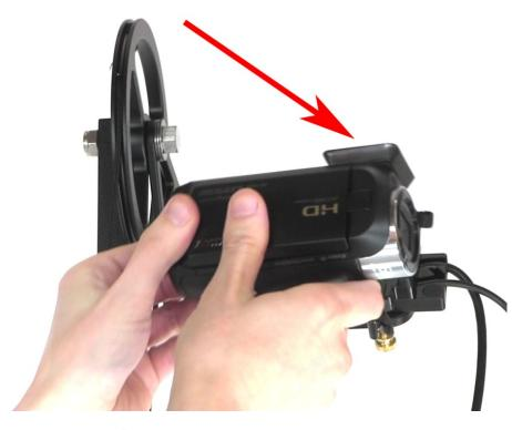
Notice how the camera already has a connection adapter attached to it. This is what you'll use to snap the camera to the quick release plate.
