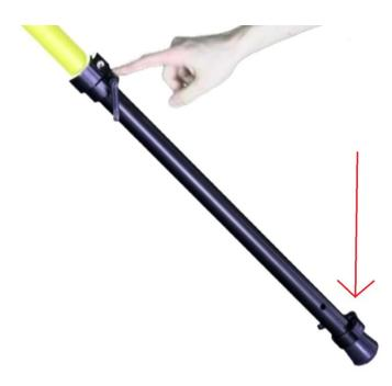
Once unlocked this allows the inner leg to extend and move freely. After extending the leg, turn the ratchet to lock. Now it is time to use the redundant safety lock. Loosen the ratchet on the safety lock, making it easy to slide. Push the safety lock up so it makes contact with the top racthet lock. Once you have done this, secure both locks tightly. Repeat this on all legs. Examine the balance bubble. You may have to adjust the legs to achieve perfect balance. (See Below)
