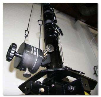
tube. Then, with the X screw simply tighten the handle mechanism clamp. As you spin the X screw you are squeezing the clamps against the
