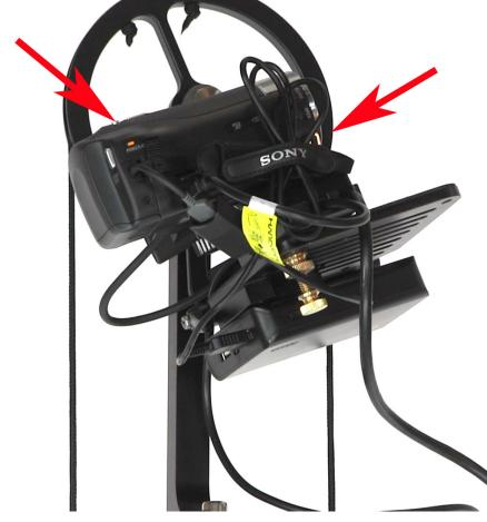
Then bind of the excess cable length of the USB adapter, and bind it inside of the camera hand-strap. This keep the cable clean and out of the way so it won't catch on anything during operation.
