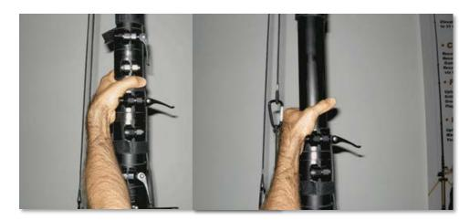
There are 5 collars for the 6 HI-POD tubes, each collar squeezing the upper tube. When you reach the recommended height you will see a white line. This white line tells you to stop elevating and lock the collar. It is not possible to push the innermost tube so high that it comes out. There is a built in safety catch that prevents the tube from coming out.
