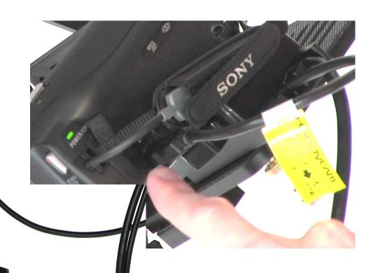
For that last step in the core cable setup, find the carabineer that is attached to the cables.
