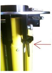
**IMPORTANT:** If you decide to split the base into three parts, when you put it back together you must make sure that the middle cylinder is locked to both the base plate (right), and to the leg bracket (left) – each secured by a twist lock.
