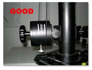
This clamp extends from the ropes that are tied to the pulley at the top of the HI-POD Tubes. You will notice these ropes fall from either side of the pulley wheel. *Remember: the ropes should come from opposite sides of the pulley wheel (just like the cylinder below)*.
