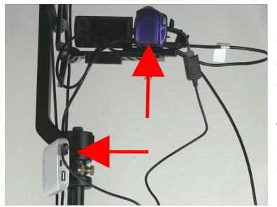
Connect the battery pack to the camera with a USB extension cable (included in your case). Note the shorter USB cable in the hand-strap of the camera, and use the longer extension to connect the camera/battery.
