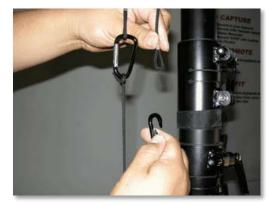
**Connecting:** As you face the HI-POD Handle, make sure the large silver screw & ropes are pointed towards the ground. Now, grab the rope that is closest to the tube. Pull that rope towards you. It will extend from the cylinder. Pull approximately 1 foot of rope, making sure that the large screw is still pointing down. With your other hand grab the other rope. Make sure this second rope is extending from the opposite side of the cylinder. Pull out the same amount of
