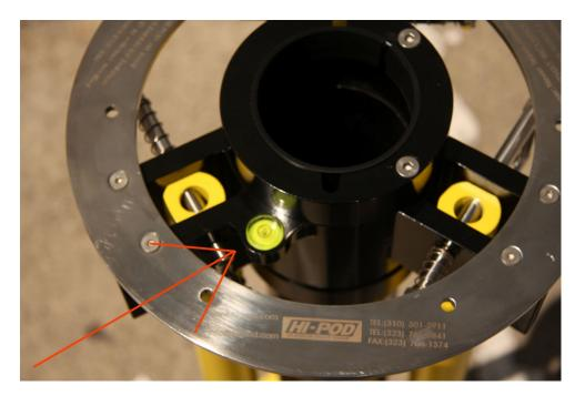
Always check the leveling bubble when setting up the HI-POD. The bubble must be level and the legs must be locked and solid.
