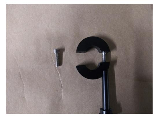
Tighten to the point where there is some mobility in the arm. Screw in bottom screw, and adjust placement of arm.
