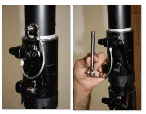
We have added an additional safety mechanism. Each locking collar for the tubes has the ability to receive a locking safety pin.
