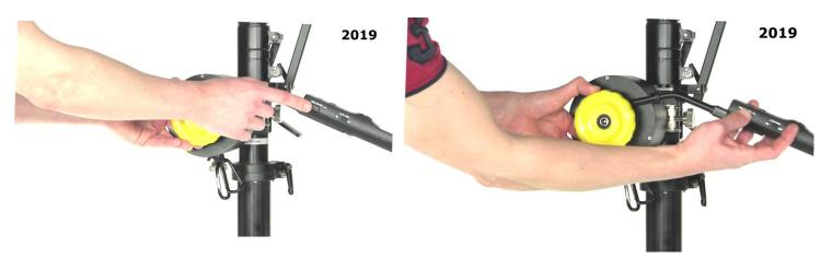
If you ever want/need to change the physical position of the remote, as it attached to the handle, you'll need to find an allen key (metric), open the screws, adjust the angle to your preference, and tighten again.
