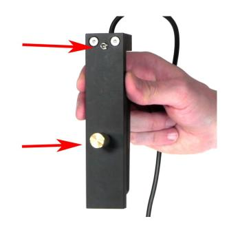
Note on the back of the remote strain relief that there is a small silver pin at
