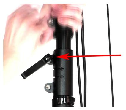
Note the lever (camlock) which you'll use to release and lock the tube collars. Repeat this for all stages.
