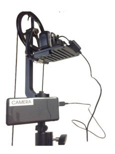
First, mount the battery to the tower (either to the top of the poles as shown or to the camera plate). Connect the battery to the camera with the female-to-male USB cable extension. The female end will connect to the USB cable found in the camera hand strap.
