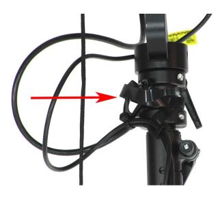
Then take the extra velcro and attach it around the tubes several times to keep it out of the way. This finishes mounting the cables, remote, and camera to the physical structure - with strain reliefs at each point.
