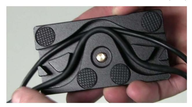
You use this plate by threading your video and lanc cables through it (in opposite directions to come out on the appropriate sides of the camera).
