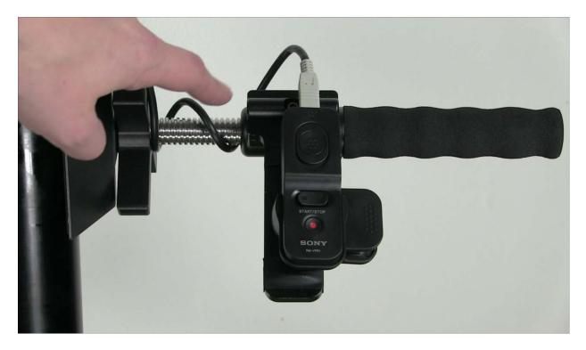
\*\*NOTE the black end of the cable plugs into the camera 'Multi' port.
