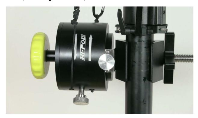
Connect the ropes coming out of the handle to the matching shorter cords coming down from the Hi-Pod Head. This engages the system. Connect with the attached carabineers.
