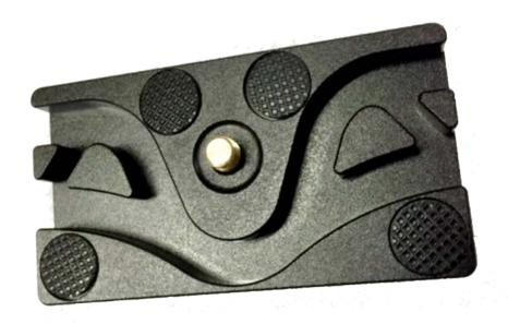
The Strain Relief Plate locks the video and lanc cables firmly under the camera. When the unit is fully elevated, it prevents gravity from pulling down on the delicate cable tips/camera ports, which can cause the tips to break or ports to widen. If damage occurs your control/video signal will drop - so **USE THIS ITEM EVERY TIME.** \*Damage to the system can occur as quickly as a single use if not applied.
