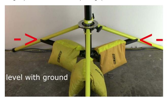
Once the black slats are level, hold them in position with the three yellow safety collars (see below). Once in place, these yellow collars will hold your leg position, while allowing the black knobs to stay unlocked, allowing the pole to turn.
