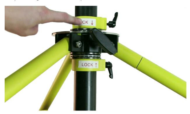
You will need to adjust this on all three yellow collars. Test when setting up the base to make sure you can turn the black pole 360 degrees with no interruption. A normal setting would place the tips of the ratchets:
