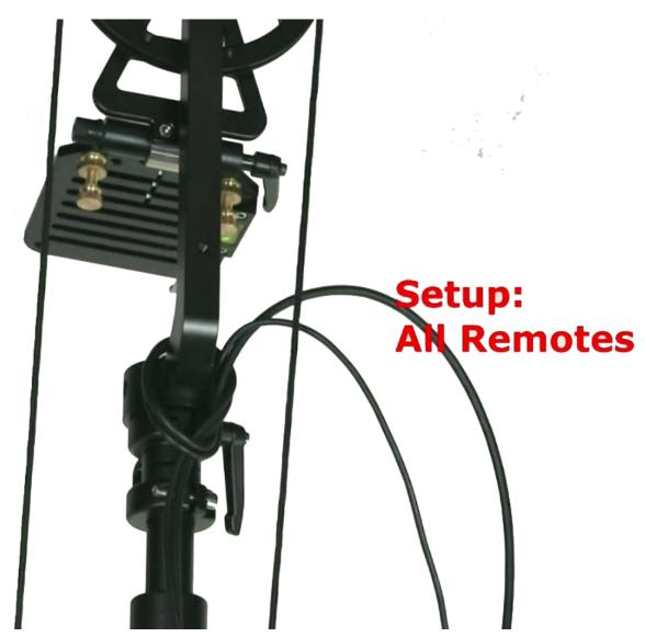
After the Strain Relief Plate is attached, to mount to the Hi-Pod wheeled head, find the smaller of the two holes next to the bottom of the brass screw. This will connect with the camera mounting screw.
