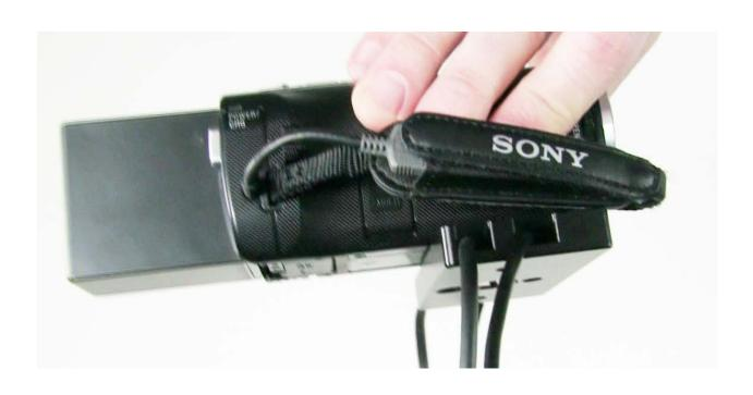
• Before mounting the camera to the wheeled plate, make a slack knot in the cables around the 'L' shape of the head, where it attaches to the tubes. This helps to cut down on cable droop, etc - just make sure to leave enough slack for the wheel/head so it can move in all directions (including straight up and down). - If you don't leave enough slack you can a damage the cables when the head begins to move.
