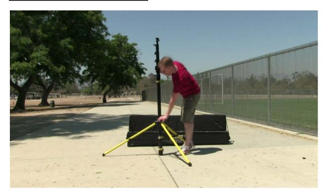
Take the tower out of your case, and place it on the ground. There are two black twist knobs on the base of the tower, and you will need to unlock these to allow for the tower legs to expand.
