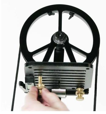
Take one of the brass camera mounting screws (attached to the plate of the head), and insert from below the plate with grooves carved out of it. You'll likely need to use one of the most exterior slots to mount.
