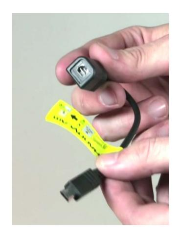
• (2) The 'Sony D-Cable' will plug into the D-shaped port on the 'Multi-Cable'. In the vast majority of cases, the only cable involved is the black cable with the stereo tip. The RCA cables are only involved if not using HDMI. Just ignore them.
