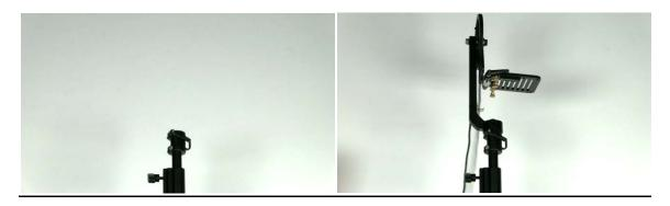
Once in place, use the ratchet at the top of the tubes to tighten and secure.
